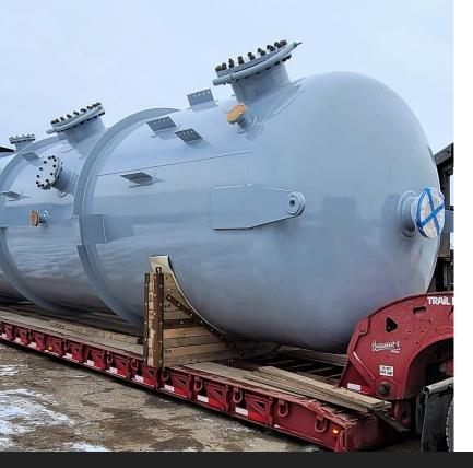
The product was applied via brush because of the complex internal geometry but the long overcoating time, allowed the applicator to complete the application successfully without the need for additional surface preparation between coats,
